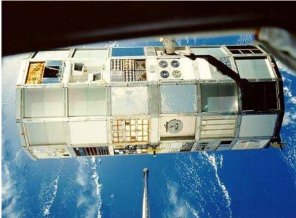
Fig. 16 Long duration exposure facility (LDEF) during the retrieval by the US space shuttle
