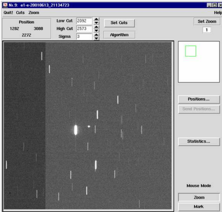
Fig. 26 Enlargement of a part of a search frame showing a 12th magnitude GEO object (point-like image at center). Stars produced trailed images in this 2-s exposure. The Figure shows about 1/16 of the entire field of view
