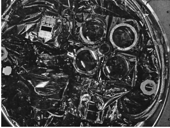
Fig. 21. MLA installed on the MESSENGER instrument deck.
