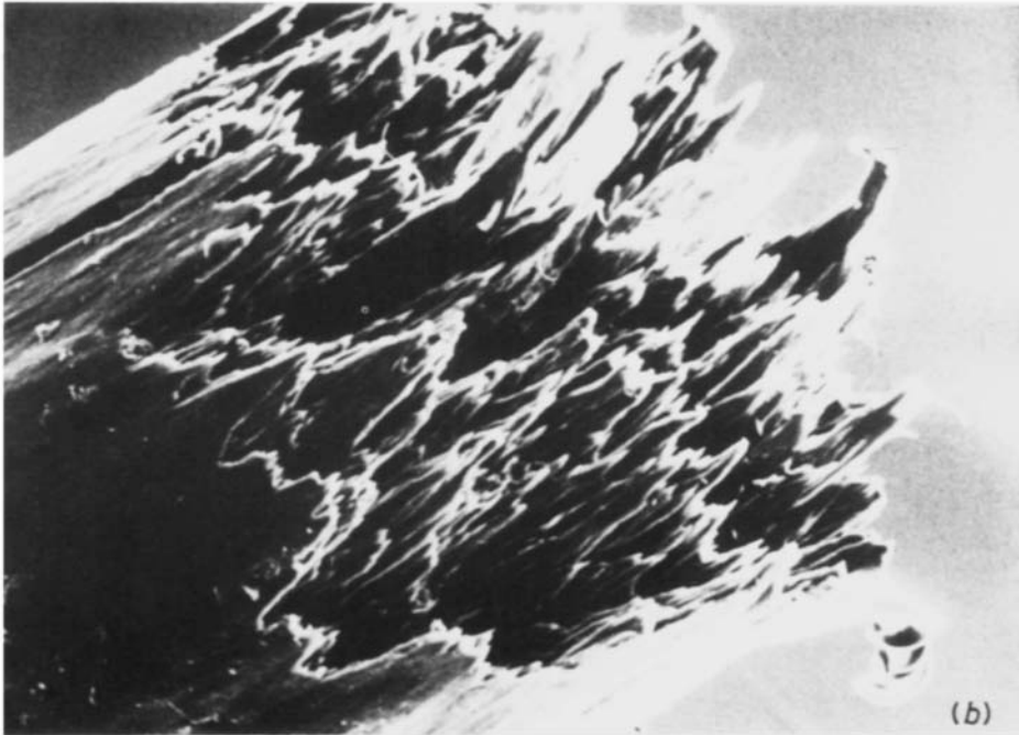
Plate 12. Scanning electron micrograph of fracture surface for polymer A5, extruded from a 1 mm die: (a) free-fall fibre of 1 mm diameter and (b) drawn-down fibre of 0.3 mm diameter.
