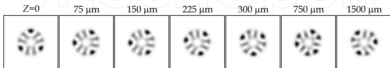
Fig. 5. Propagation of a superposition of (p, q) : (2, 2) + (-4, 1) + (5, 1) : transverse distributions of intensity at different distances z .
