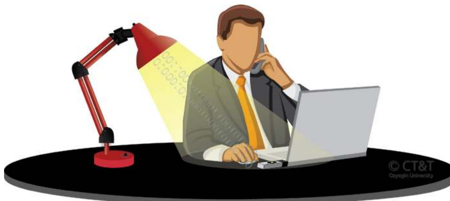
Figure 5. A VLC-enabled hot spot where the VLC receiver in the form of an USB dongle communicates with the desk lamp acting as a VLC transmitter.
