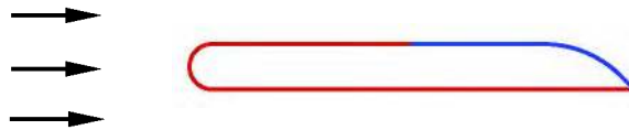
Figure 1: Blake airfoil used in unsteady laminar flow problem. The right half section of the upper surface is allowed to deform.
