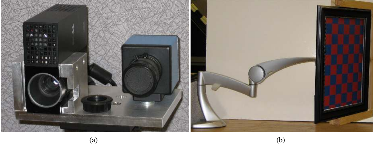
Fig. 2. (a) Photograph of the 3D shape measurement system; (b) Photograph the universal mounting frame to hold calibration board.
