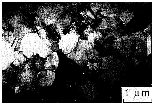
Fig. 14. Transmission electron micrograph of 16Cr–10Ni steel annealed at 873 K for 0.6 ks after 90% cold rolling, showing ultra fine austenite grains with a mean size of 0.5 \mu\text{m} .
