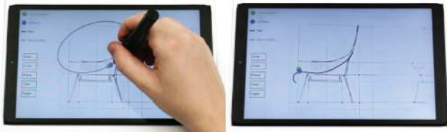
Figure 11. Virtual tools can be used to dynamically construct a reference path combining haptic and visual feedback. Here a simple drawing application combines freeform sketching with different virtual rules and guides that can be felt by the user.
