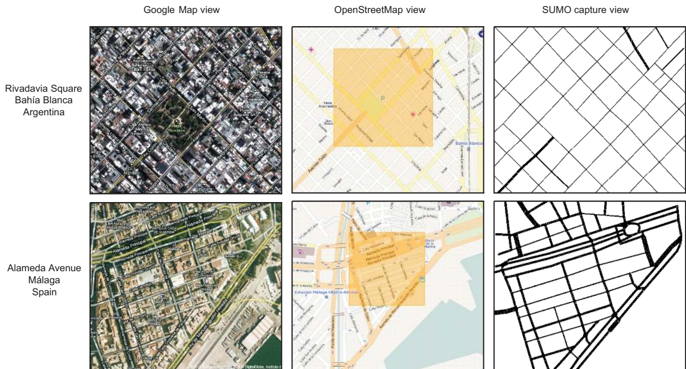
Fig. 3. Process of creation of real-world instances for study. Rivadavia Square ( 38^{\circ}43'03''S 62^{\circ}15'56''O ) and Alameda Avenue ( 36^{\circ}43'60''N 4^{\circ}25'87''O ) instance views. After selecting our area of interest (Google map view), it is interpreted by means of the OpenStreetMap tool, and then exported to SUMO in XML format
