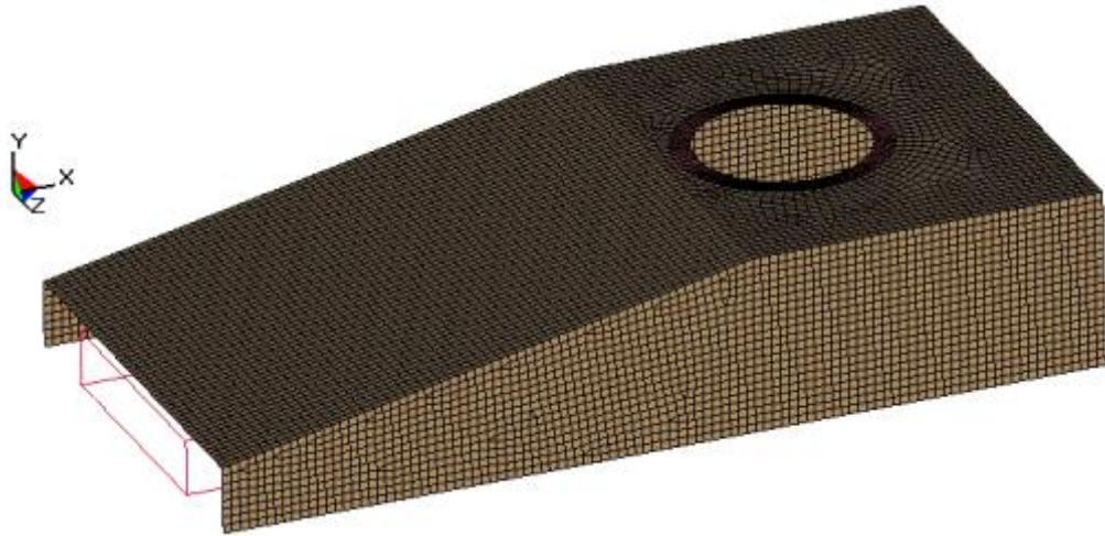
Figure 3.1: FE model of the vehicle with the internal space frame
