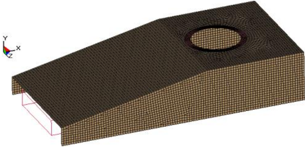
Figure 5.4: FE model of the vehicle with the internal space frame structure
