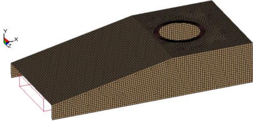
Figure 2.11: FE model of the vehicle with the internal space frame
