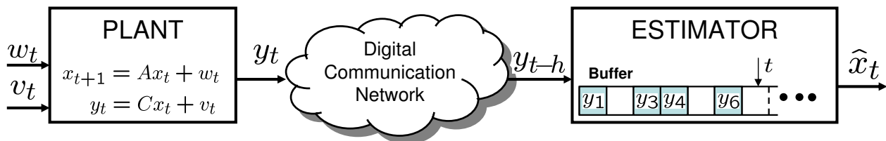
Fig. 2. Networked systems modeling. Sampled observations at the plant site are transmitted to the estimator site via a digital communication network. Due to retransmission and packet loss, observation packets arrive at the estimator site with possibly random delay.
