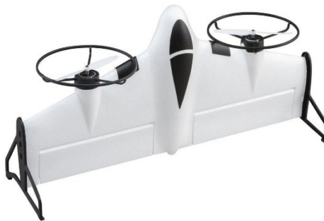
Figure 1: A tail-sitter VTOL UAV Aircraft [4]
