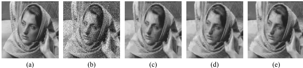
Fig. 13. (a) Original Barbara image (intensity range [0.93, 15.73] ), (b) Poisson-count image, (c) image denoised with BM3D and the exact unbiased inverse (average NMISE = 0.0881 and PSNR = 25.92 dB), (d) image denoised with BM3D and the MMSE inverse with the oracle Monte-Carlo estimate \epsilon_{MC} (average NMISE = 0.0971 and PSNR = 25.80 dB), (e) image denoised with BM3D and the MMSE inverse with the SURE estimate \epsilon_{SURE} (average NMISE = 0.0911 and PSNR = 25.91 dB).
