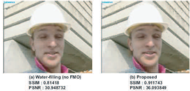
Fig. 4. Reconstructed Image of (a) WF (without FMO), (b) Proposed Scheme (with FMO). SNR=2dB.
