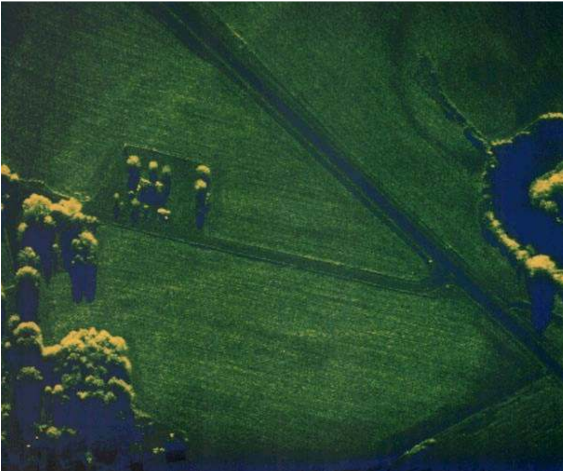
Fig. 6—SAR image of farm area ( 1\text{-m} \times 1\text{-m} resolution) corresponding to aerial photograph shown in Fig. 5. This image was formed by first applying PWF processing to the 1-ft coherent data, then spoiling ( 4 \times 4 noncoherent averaging) to an effective 1-m resolution.
