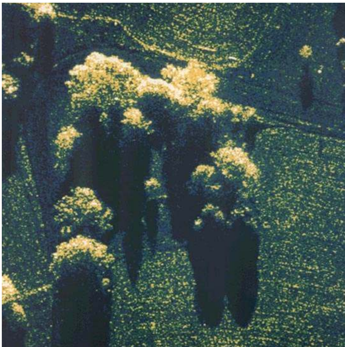
Fig. 7—PWF image of trees (1-ft \times 1-ft resolution). This image, taken from an area near the farmhouse, shows the detail obtained from PWF processing of ADTS data. Note the bright leading edges of the trees and the radar shadows directly behind the trees.
