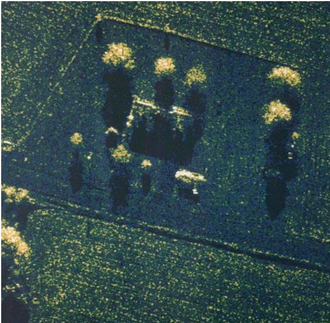
Fig. 1—ADTS SAR image of farmhouse in Stockbridge, N.Y. (1-ft \times 1-ft resolution). The sensor was flown at an altitude of 2 km with a look-down (depression) angle of 22.5°, giving a slant range of 7 km. PWF processing was used to produce this minimum-speckle image. The radar is located at the top of the image, looking down; therefore, the radar shadows go toward the bottom of the page.
