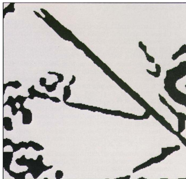
Fig. 12—Segmented version of PWF farm image (shown in Fig. 6) into two clutter types: bright and dim.
