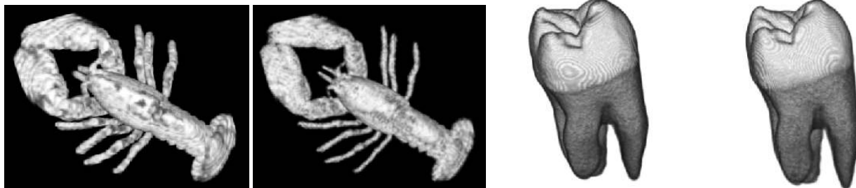
Figure 1: CT scans of a lobster and a tooth, represented on Cartesian and body-centered cubic grids (left and right images, respectively). The representation via body-centered cubic grids requires approximately 30% less samples.
