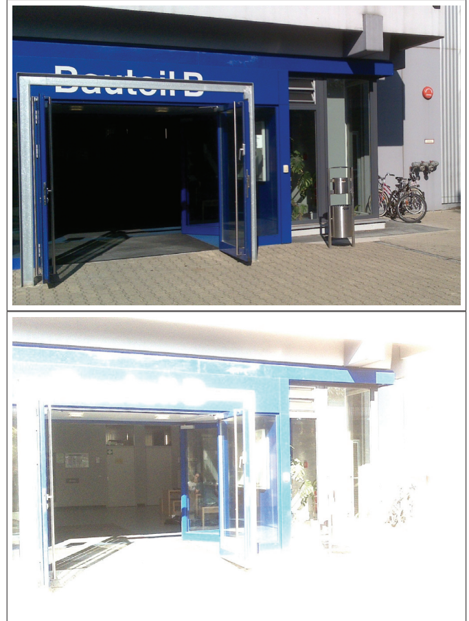
Fig. 1. The inside of the building is much darker than the outside. There is no shutter speed setting that exposes both correctly at the same time. A solution to this problem is using a sequence of shutter speeds and merging the images together.
