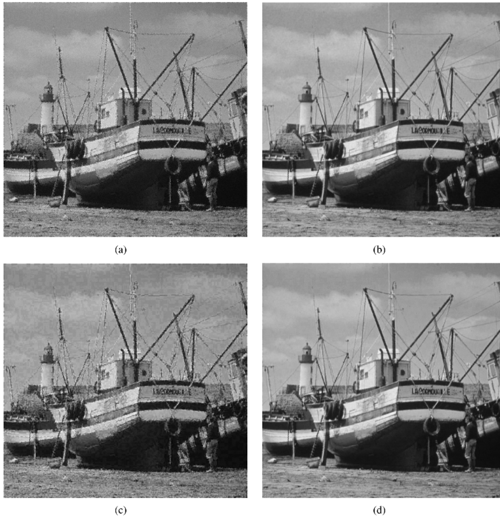
Fig. 3. Watermarked versions of the Boat image obtained for the four different optimization formulations. (a) Maximizing embedding strength. PSWR of the image is 24.60 dB. (b) Minimizing frequency weighted perceptual distortion. PSWR of the image is 37.71 dB. (c) Maximizing robustness to compression. PSWR of the image is 24.79 dB. (d) Minimizing the watermark texture visibility. PSWR of the image is 37.28 dB.
