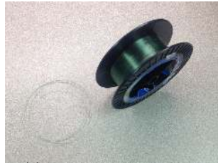
(c) Fishing line cable with 20 lb maximal payload.
