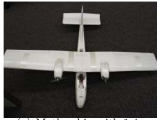
(a) Mothership with 1.4 m wing span, twin props and cable release mechanism.
