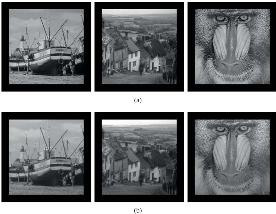
Figure 2.2. (a) Different \mu_1 distributions for a fixed source \mu_0 . (b) Ray-tracing resimulation via Monge–Ampère computation of the reflector. Figure reproduced from Brix, Hafizogullari and Platen (2015) with permission. Copyright © 2015 World Scientific.
