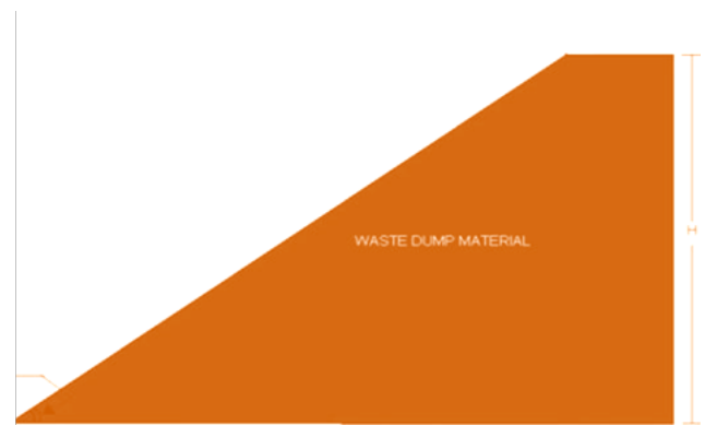
Figure 1. General Geometry of dump slope with Height, H = 60\text{m}
