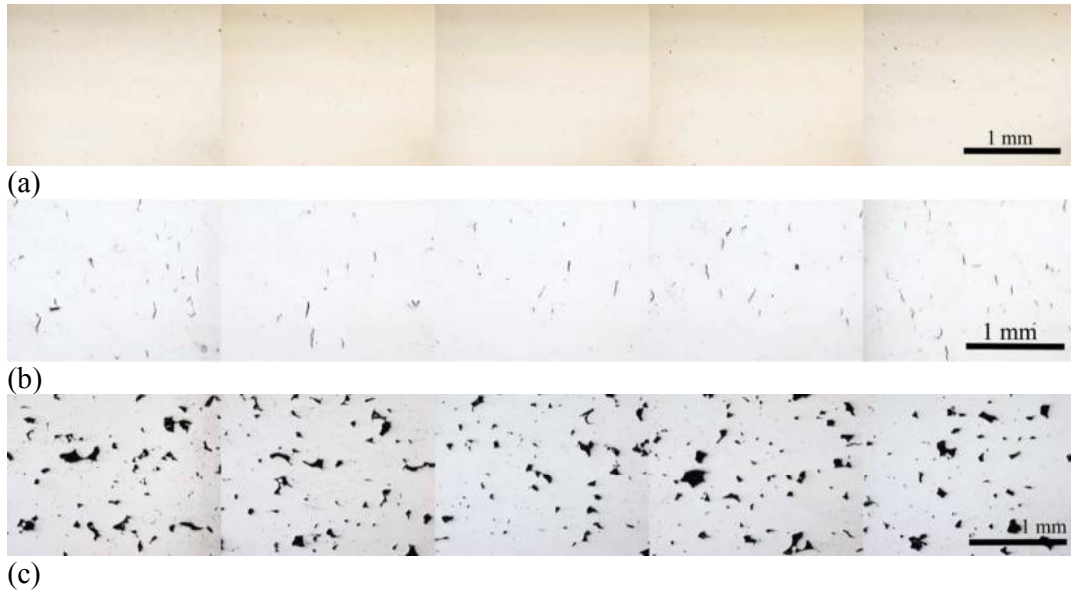
Figure 9: Optical micrographs of ground and polished surfaces of IN-738 LC (a) 270 W, 1084 mm/s and 0.09 mm; (b) 345 W, 850 mm/s and 0.11 mm and (c) 295 W, 2250 mm/s and 0.11 mm SLM processing parameters.
