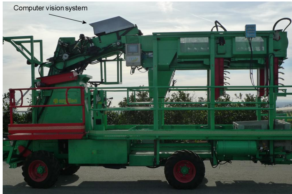
338 339 Figure 8. Mobile platform with the grading system
