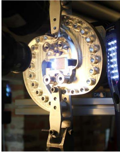
Figure 20: Short Off-axis Tensile (SOT) test experimental set up.
