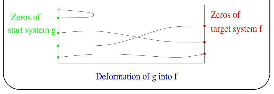
Complete motion synthesis for so called Stephenson mechanisms can be performed efficiently by homotopy methods
