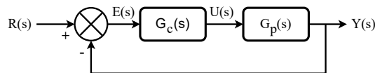
Figure 2. Classical control diagram to regulate voltage in the buck converter of Figure 1.
