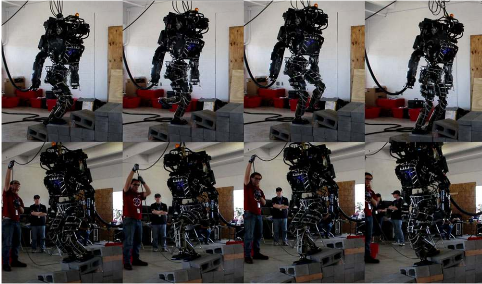
Figure 6. These photos show the Atlas robot practicing for segment 3 of the terrain task for DRC. The snapshots were taken every 5 s
