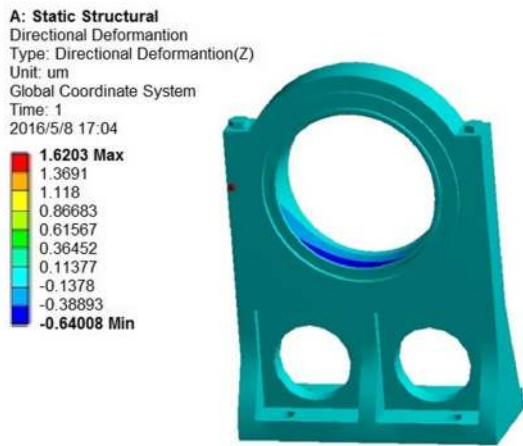
c deformation nephogram of the left mount
