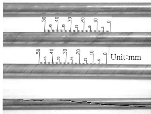
**Figure 1:** Roll marks and section crushing of an Al7001T9 pipe.
