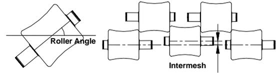
**Figure 3:** The slanted angle and the intermesh of roller.
