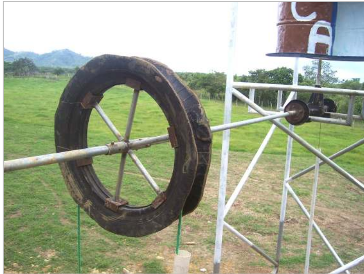
Figure 4: Pump wheel constructed from truck sidewalls of truck tires with a welded steel hub.
