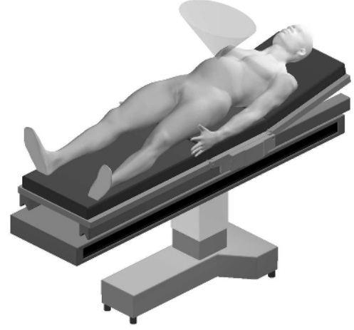
Fig. 4. Workspace in MIS: an elliptical cone with vertex angles of 60^\circ and 90^\circ represents the workspace such that the endoscopic tool can reach any organ in the abdomen. The ports are placed such that the end-effector of the tools can access the target anatomy. In this illustration, the port is located at the center of the abdomen with the cone at 90^\circ elevation.
