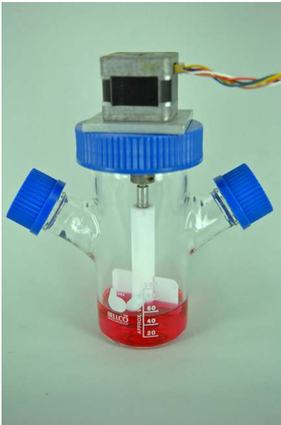
Fig. 1 Spinner flask set up with the impeller directly connected to a stepper motor
