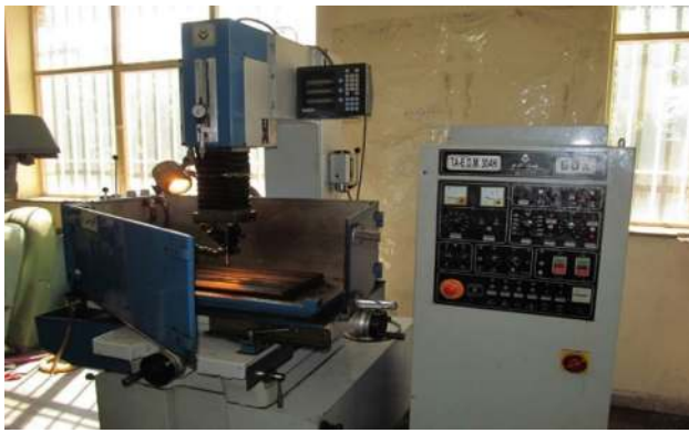
Fig. 2 The Azaraksh-304H EDM machine used for conducting experiments
