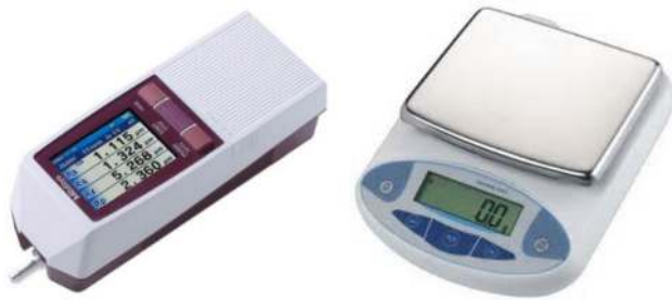
Fig. 3 The electronic balance and surface roughness tester used
