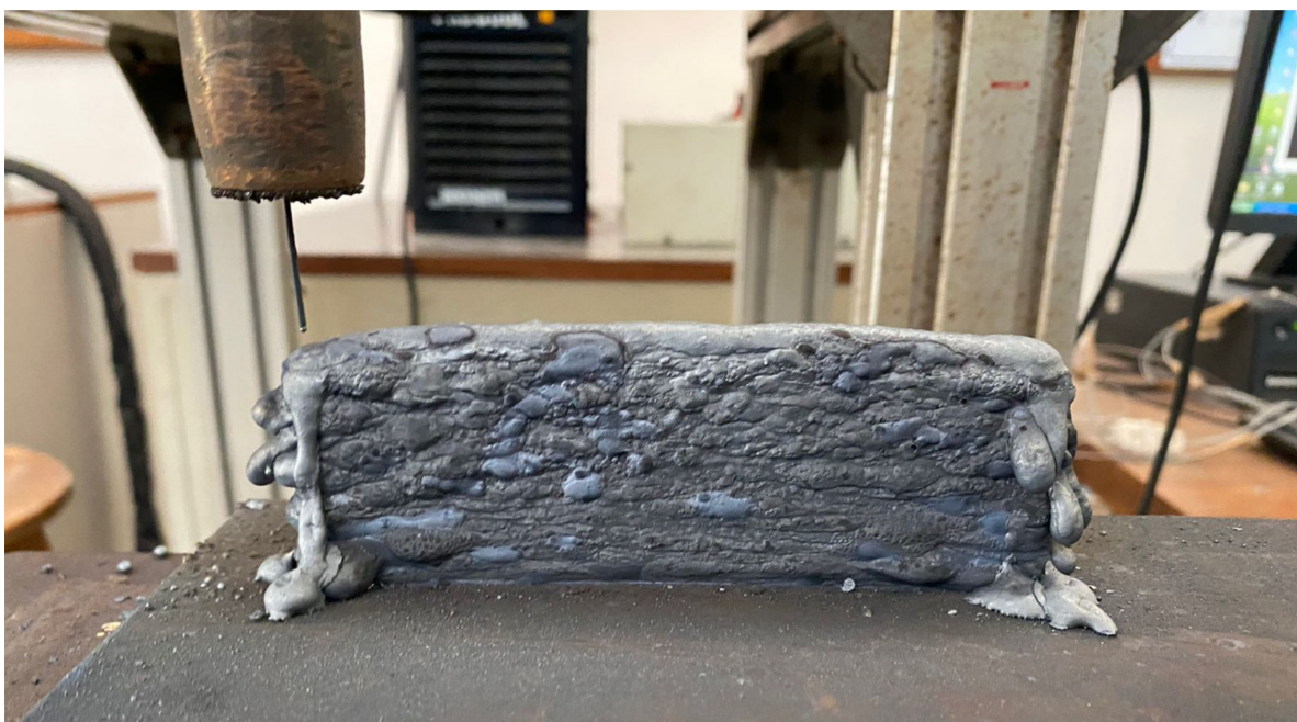
Figure 10. Multi-layer structure obtained at optimized parameters.
