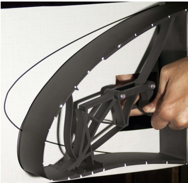
Figure 28. Experimental test for the identification of the maximum deflection shape corresponding to a 70 deg rotation of the shaft.
