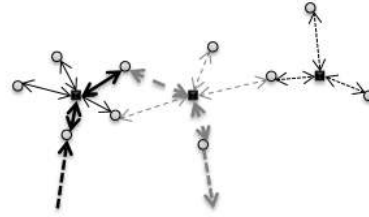
(b) The same three services in an service flow formulation. The service nodes are added in the middle of the three services, which then are connected with their called ports by arcs, opened by binary variable \theta_{i,b,s} and flow by continuous variable f_{i,b,s}^k . A flow path entering the first service, transshipping for the second and unloading at the flow destination is shown.
