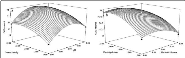
Figure 4 Response surface plots (3D) for the effects of variables on the COD removal. (a) Effect of pH and current density (b) Effect of electrode distance and electrolysis time.
