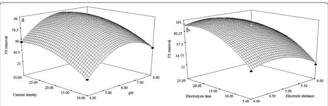
Figure 3 Response surface plots (3D) for the effects of variables on the TS removal. (a) Effect of pH and current density (b) Effect of electrode distance and electrolysis time.
