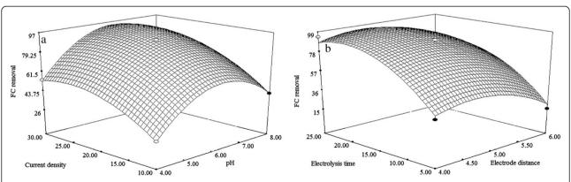
Figure 5 Response surface plots (3D) for the effects of variables on the FC removal. (a) Effect of pH and current density (b) Effect of electrode distance and electrolysis time.
