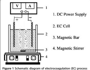
Figure 1 Schematic diagram of electrocoagulation (EC) process unit.
