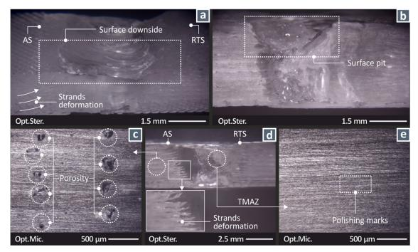
**Figure 5.** Views of the welded specimens' side (vertical) surface (the weld tool performs the weld on the top surface): (**a**) HAZ stereoscopic image (1000 rpm, 6 mm/min, PPA); (**b**) HAZ stereoscopic image (1400 rpm, 6 mm/min, PPA). Specimen welded at 1000 rpm, 3 mm/min, PPA: (**c**) view outside the welding zone, (**d**) stereoscopic image, and (**e**) view of the welding zone (AS: advancing side, RTS: retreating side, TMAZ: thermomechanically affected zone).
