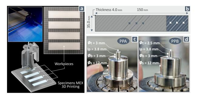
**Figure 1.** (a) MEX 3D-printed specimens for the FSW process; (b) specimen dimensions and infill pattern (lines and arrows indicating the specimen's 3D-printed structure); (c) Welding Tool A (PPA) dimensions; (d) Welding Tool B (PPB) dimensions.
