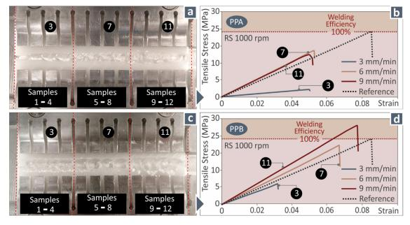
**Figure 4.** (a) PPA welding tool's weld seam; (b) stress–strain graphs from the tensile tests for the different TS values (RS 1000 rpm, PPA); (c) PPB welding tool's weld seam; (d) stress–strain graphs from the tensile tests for the different TS values (RS 1000 rpm, PPB).
