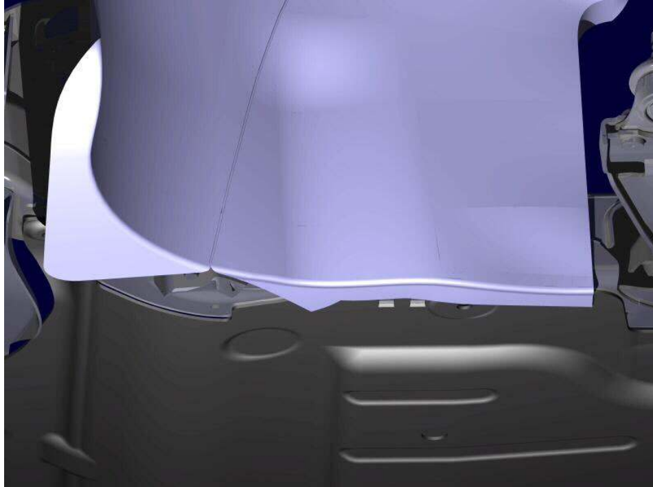
Figure 66 Picture of the covered gap, the dark grey part at the bottom of the picture is the under-shield
