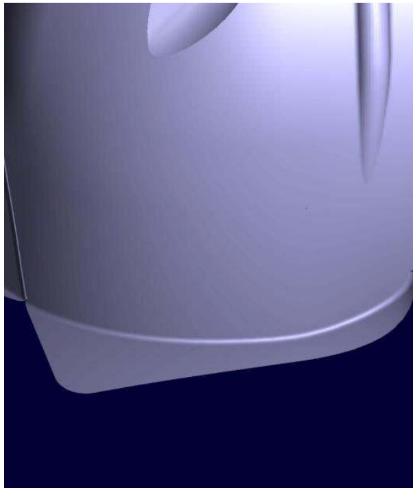
Figure 61 Folded edge, picture taken at the bottom, at the front part of the wheel arch liner
