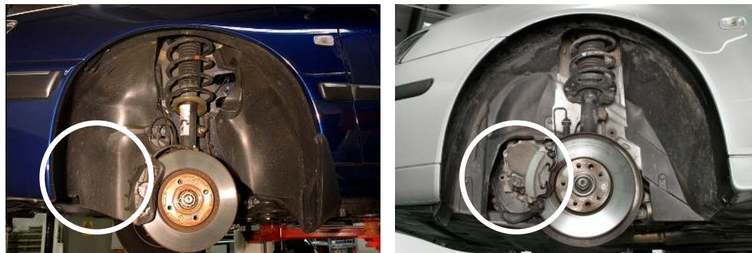
Figure 9 With splash shield, Peugeot 406, respectively without splash shield, SAAB 9-3
