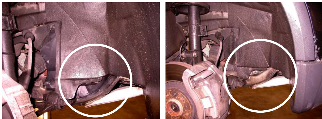
Figure 10 XC90 with and without splash shield
