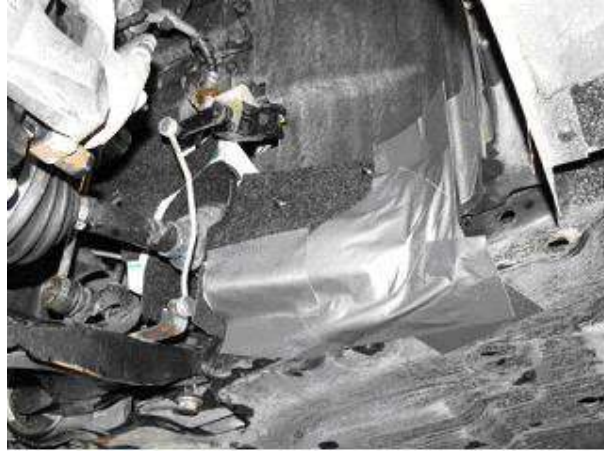
Figure 13 Contamination test with a splash shield attached to the under-shield
