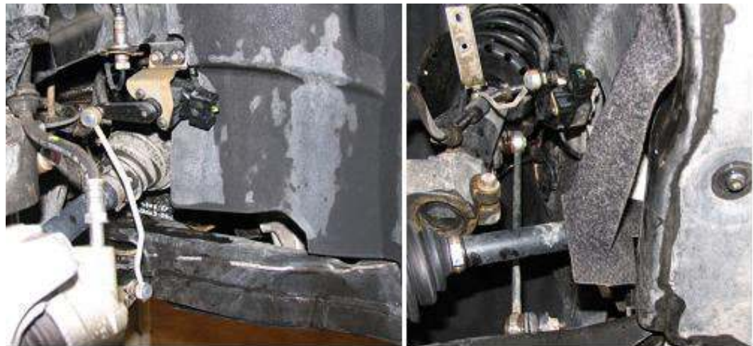
Figure 12 Contamination test without splash shield and with a home made splash shield
