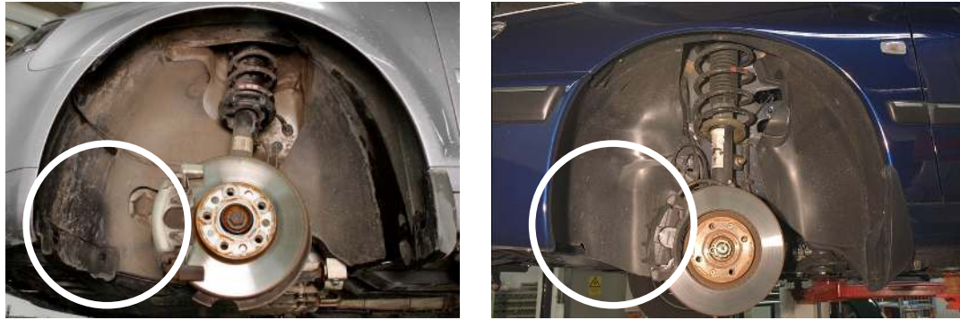
Figure 8 Splash shield integrated in the wheel arch liner, Audi A3 respectively Peugeot 406
