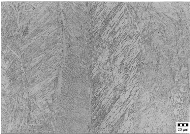
Figure 7: Microstructure of weld metal in the middle of weld nugget of sample B.
