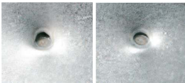
Figure 4: Failure of the spot welds after tensile test: a) H260 steel, b) H340 steel.
