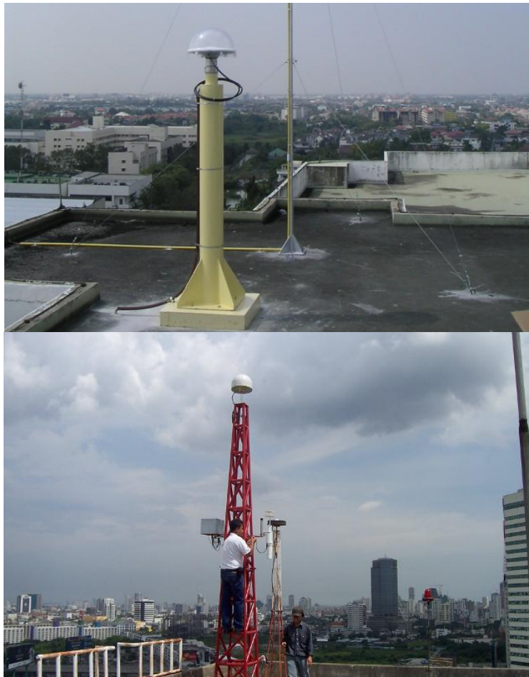
Fig. 5. Top: The PKKT station (base station), Bottom: The DPT9 station (roving station)
