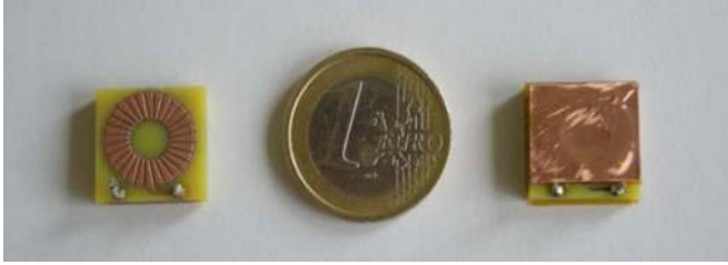
Fig. 14. Prototypes of 500 nH PCB air-core toroid without and with shield.
