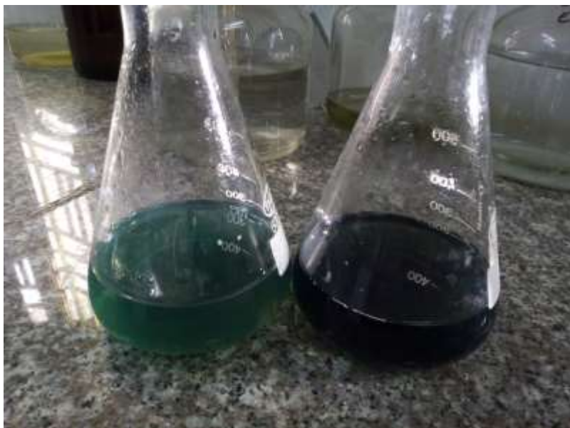
Figure 2. End point of a reaction using 15 drops of diphenylamine indicator (at the right) and using 8 drops of diphenylamine indicator (at the left) for similar soil sample.
