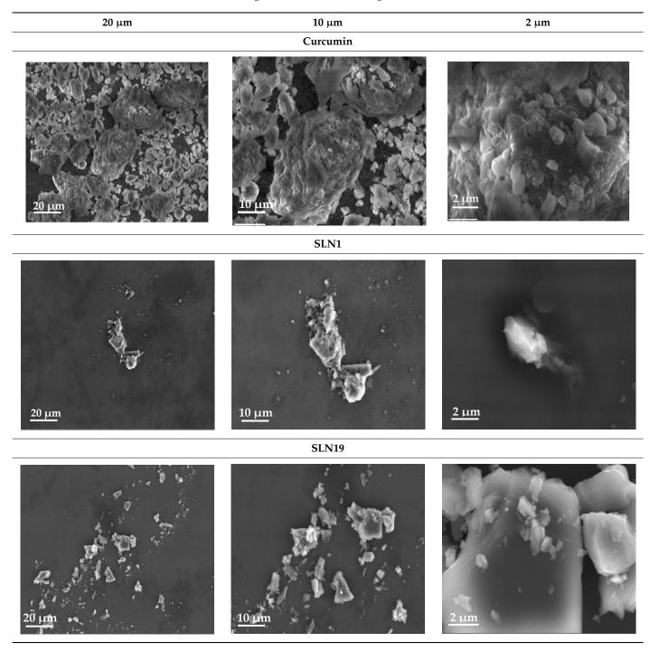
Table 3 shows the scanning electron microscopy SEM images of pure curcumin, SLN1 and SLN19. Image magnification allowed the observation of particles on a scale from
