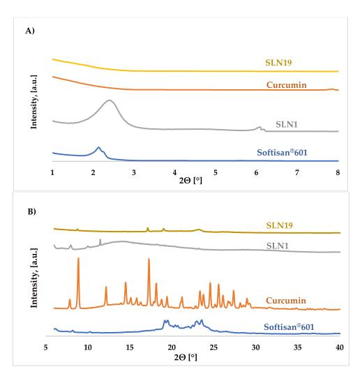
**Figure 6.** Comparison of XRD diffractograms: (**A**) low-angle diffractograms for Softisan<sup>®</sup> 601, SLN1, curcumin and SLN19, and (**B**) wide-angle diffractograms for Softisan<sup>®</sup> 601, SLN1, curcumin, and SLN19.
