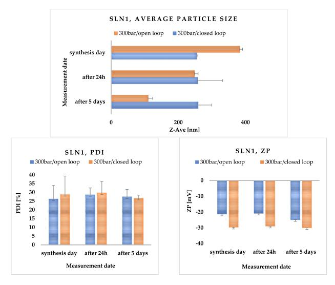
**Figure 4.** Comparison of average particle size, polydispersity index (PDI) and zeta potential (ZP) of nanoparticles synthesized with Softisan<sup>®</sup> 601 lipid and Poloxamer 188 at 300 bar, measured on the day of synthesis, and additionally 24 h and 5 days after the synthesis. The process of obtaining nanoparticles was carried out in an open- and closed-loop systems in three cycles.
