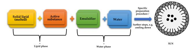
Scheme 1. Block diagram of the structure of a solid lipid nanoparticle. Based on [17].
