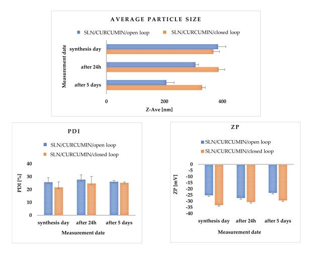
**Figure 5.** Comparison of the average particle size, polydispersity index (PDI) and zeta potential (ZP) of SLN-type lipid nanoparticles synthesized at 300 bar and incorporated with curcumin, measured on the day of synthesis, 24 h after synthesis and 5 days after synthesis, for a closed-loop system. The process was carried out in an open-loop and a closed-loop system in three cycles.
