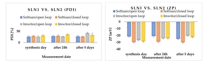
**Figure 2.** Comparison of polydispersity index (PDI) and zeta potential (ZP) of SLNs synthesized using lipids: Softisan<sup>®</sup> 601 and Imwitor<sup>®</sup> 900 and the surfactant Poloxamer 188 measured on the day of synthesis, and additionally 24 h and 5 days after the synthesis. The process of nanoparticle preparation was carried out in both open- and closed-loop systems under 300 bar pressure in three cycles.
