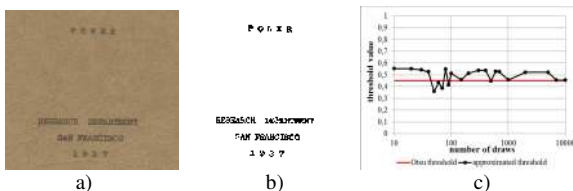
Fig. 5. Original input image PR7 (a) with “ground truth” (b) and results of threshold approximation (c) for different numbers of drawn pixels.
