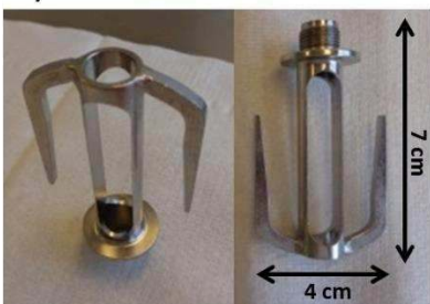
Figure 1. Digital photographs showing (a) the Chemspeed A100 automated synthesizer, (b) a 100 mL reaction vessel and stirrer module, (c) a propeller-type stirrer and (d) an anchor-type stirrer.
