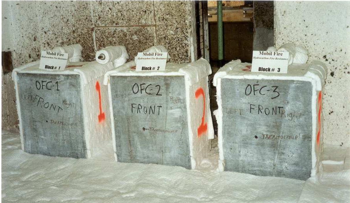
Fig.2 – View of three blocks before the hydrocarbon-fire test
