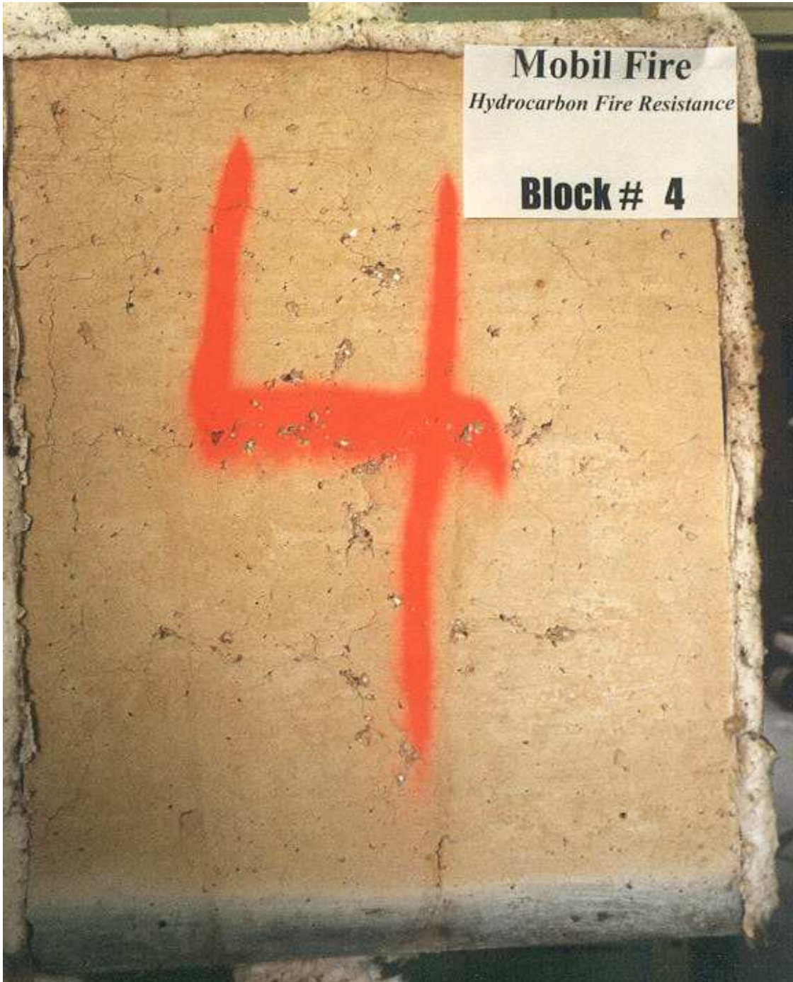
Fig. 6 – View of the Block No. 4 ( W/C = 0.33 , low-absorption coarse aggregate, 1.5 \text{ kg/m}^3 of 12.5-mm fibres) after the hydrocarbon-fire resistance test.
