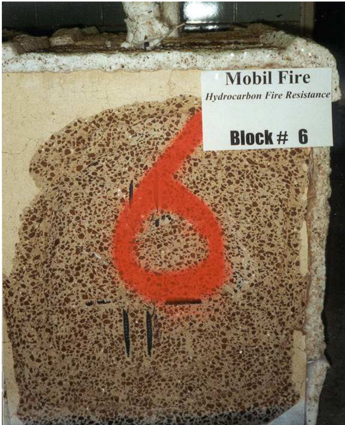
Fig. 8 – View of the Block No. 6 ( W/C = 0.33 , high-absorption coarse aggregate, 1.5 \text{ kg/m}^3 of 20-mm fibres) after the hydrocarbon-fire resistance test.
