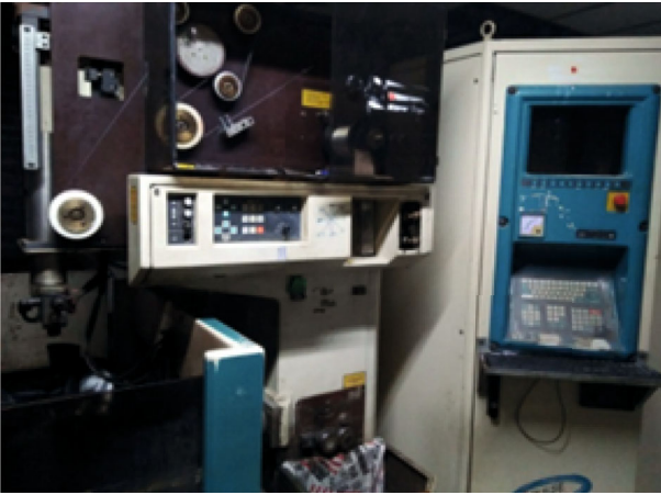
FIGURE 2: Photograph of Electronica sprint cut CNC wire-cut electrical discharge machine.
