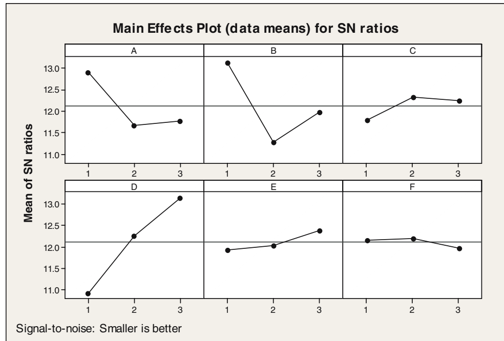
Fig. 7 Effect of control factors on kerf
